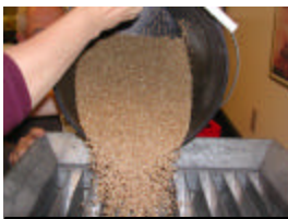
Dividing down with a riffle divider
